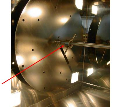
To remove the discs from the central shaft, simply unscrew the retaining nut that releases the disc for removal.
